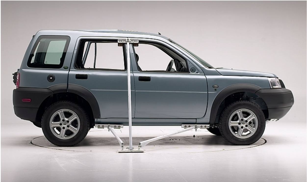
Figure 5 Antiroll Device for Tests of SUVs, Pickups, and Passenger Vans
